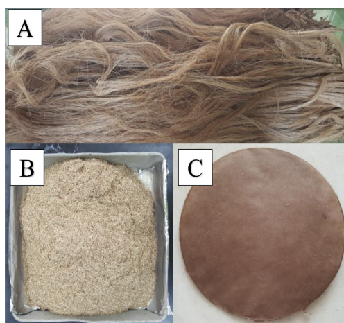
Figure 1. Bakong fibers: (a) as received, (b) after milling, (c) after hand sheet formation
